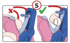
Check pin is located correctly.
